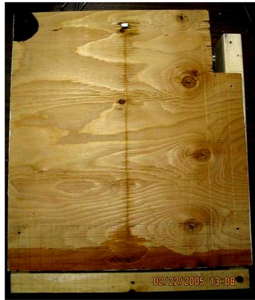
Figure 2. Wetting pattern of sheathing after 210 minutes of wetting at a rate of 12 ml/h.
