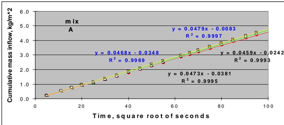
Figure 2 Initial water absorption process, measured at SU on stucco mix A.
