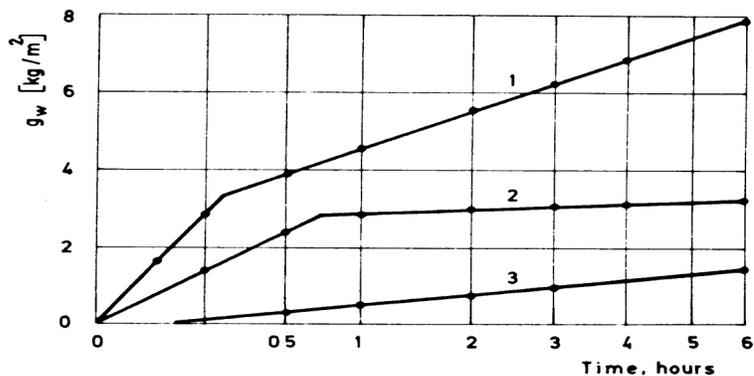
Figure 1 Cumulative water flow,  $g_w$ , to clay brick through stucco, plotted against time. Curve 1 represents lime stucco ( $A_o = 0.07 \text{ kg/m}^2\text{s}^{1/2}$ ), curve 2 is lime on a cement-splattered surface, and curve 3 is a cement stucco ( $A_o = 0.01 \text{ kg/m}^2\text{s}^{1/2}$ ). Kruger and Eriksson (1925, see Bomberg, 1974)
