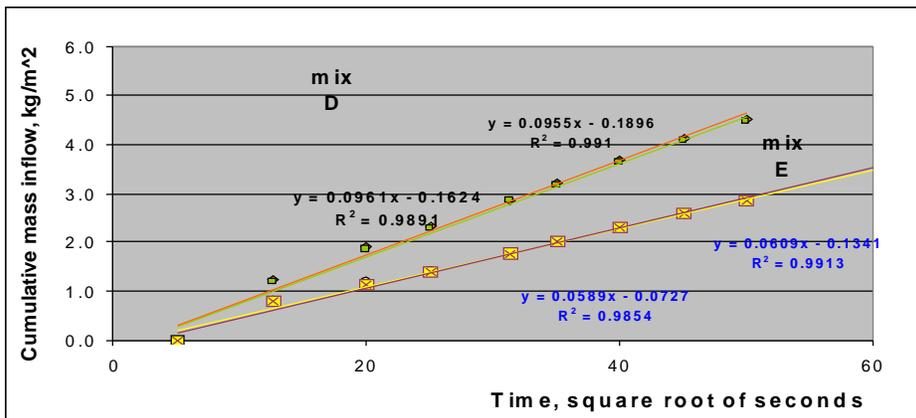
Figure 4: Initial water absorption process, measured at SU on the stucco mixes D and E.
