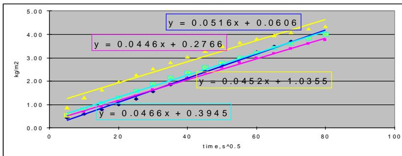
Figure 7: Water absorption coefficient measured on insulated stucco made in Beijing
