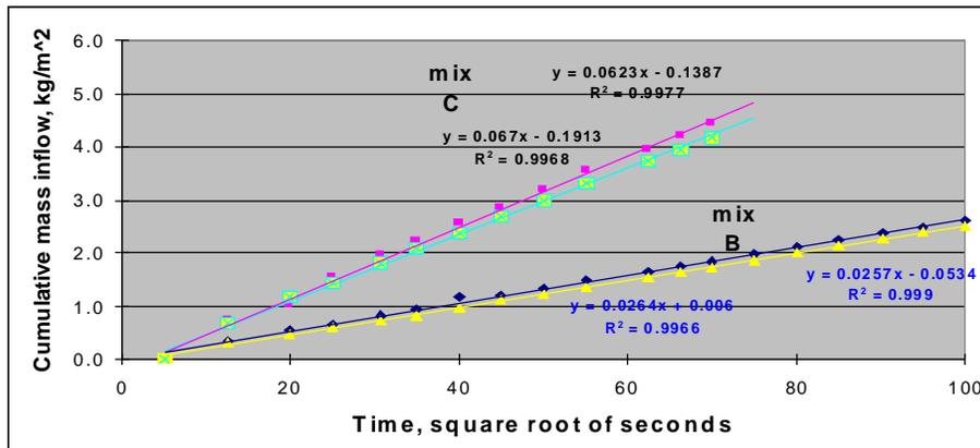
Figure 3 Initial water absorption process, measured at SU on stucco mixes B and C.
