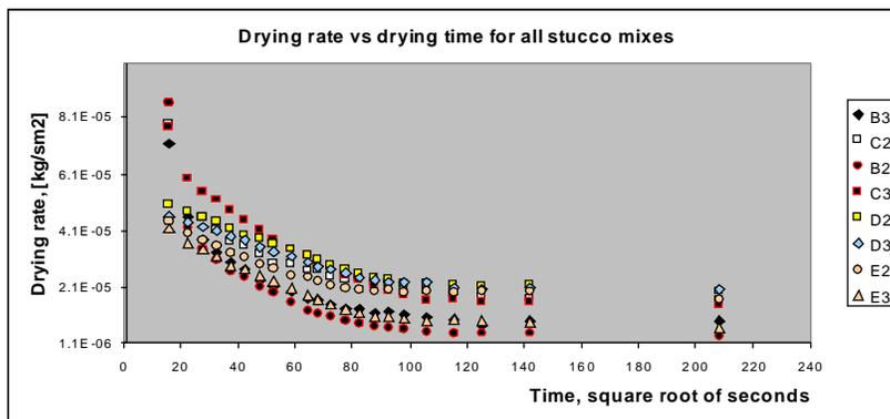
Figure 5: Drying rate versus drying time measured at SU on all stucco mixes. (The same scale is used only for comparison with wetting)
