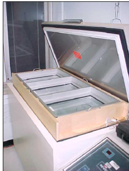
**Figure 4:** Simulated indoor / outdoor exposure apparatus designed by GRG and installed over the top of a low-temperature freezer at the Insulating Glass Laboratory at Bodycote Materials Testing Canada Inc.
