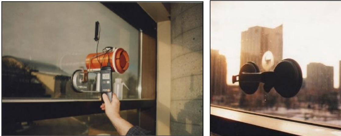
**Figures 1 and 2:** Field dew point measurement apparatus, as described in ASTM E 576. At left, the apparatus is mounted on an insulating glass unit in contact with the inboard pane of glass. A digital thermometer measures the temperature close to the glass surface. At right, the apparatus has been removed (except for the suction cups), revealing a circle of condensation or frost on the cavity-side surface of the pane induced by the chilled contact area of the apparatus.
