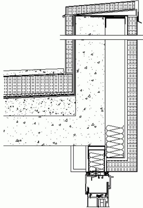
*Figure 9: Double window-wall head and sill detail*
