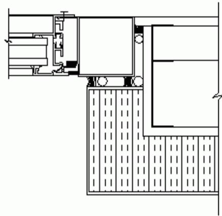
Figure 4: Existing window jamb detail
