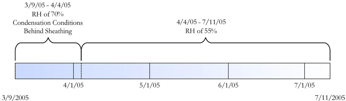
**Figure 9: Timeline for Test Number 2 – Relative Humidity Conditions on Interior Side of the Climate Chamber (Climate Side Maintained at 26°C and Relative Humidity of 80%)**
