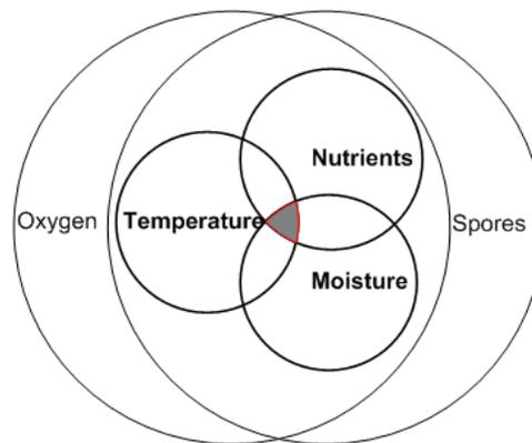
**Figure 1: Mould Growth Requirements (OAA 2003)**
