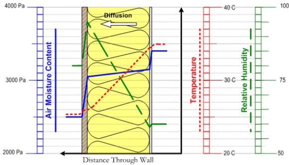
**Figure 4: 26°C & 95% Relative Humidity at Back of Sheathing**
