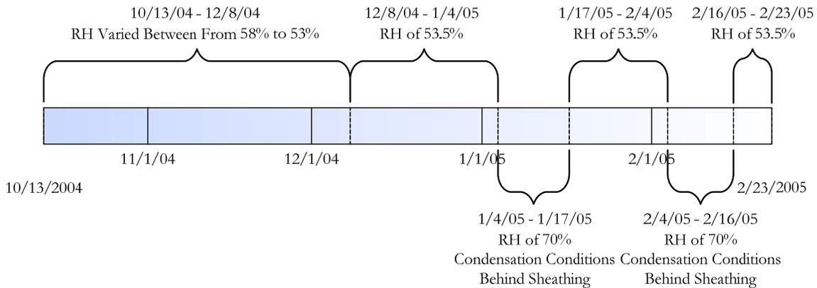
**Figure 8: Timeline for Test Number 1 – Relative Humidity Conditions on Interior Side of the Climate Chamber (Climate Side Maintained at 26°C and a Relative Humidity of 80%)**
