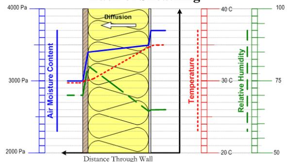
**Figure 7: 30°C & 80% Relative Humidity at Back of Sheathing**
