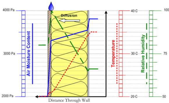
**Figure 6: 20°C & Condensation Conditions at Back of Sheathing**
