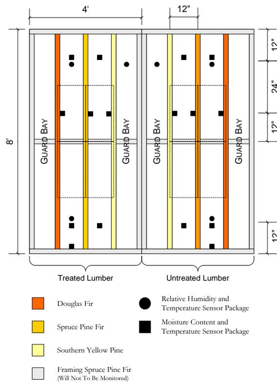
**Figure 3: Test Panel Stud Framing Layout and Sensor Locations**
