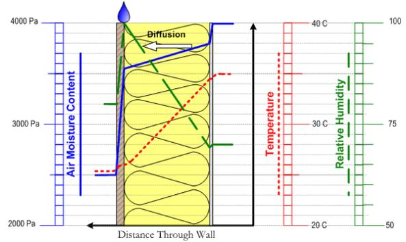
**Figure 5: 26°C & Condensation Conditions at Back of Sheathing**
