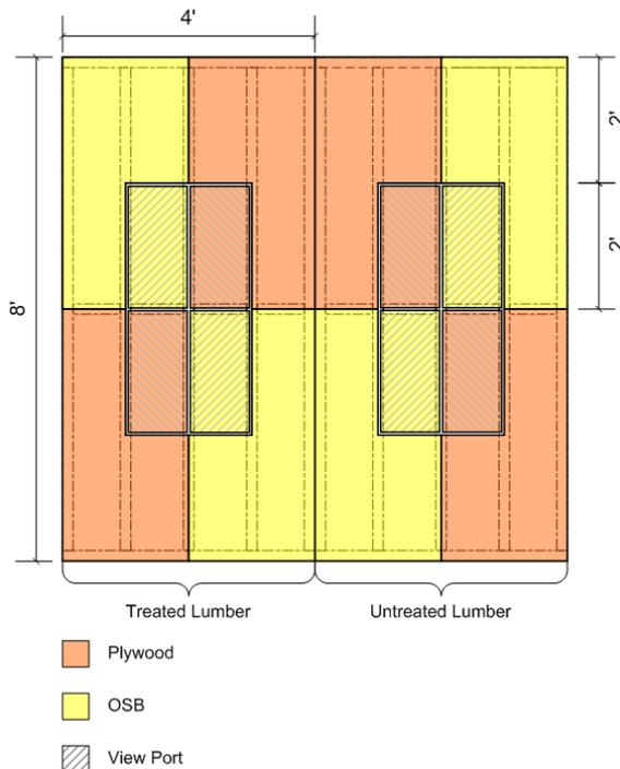
**Figure 2: Sheathing Layout of Two 4' x 8' Test Panels**
