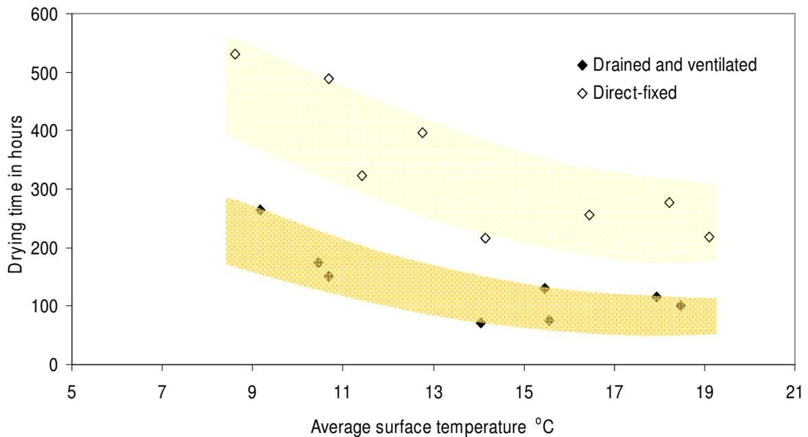
Figure 5. Drying times from insulated cavities for direct-fixed and drained and ventilated walls as a function of average cladding surface temperature.
