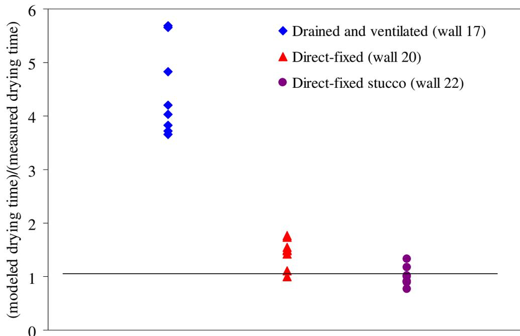
Figure 6. Ratio of modeled drying time to measured drying time for three walls.
