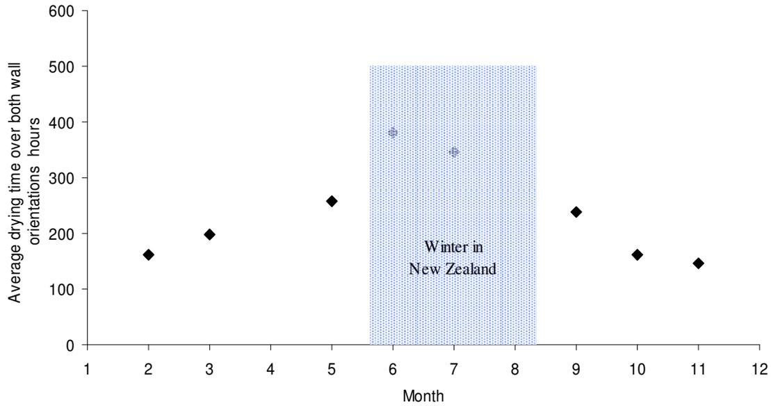
Figure 4. Seasonal changes in average drying times from insulated cavities in experimental walls.
