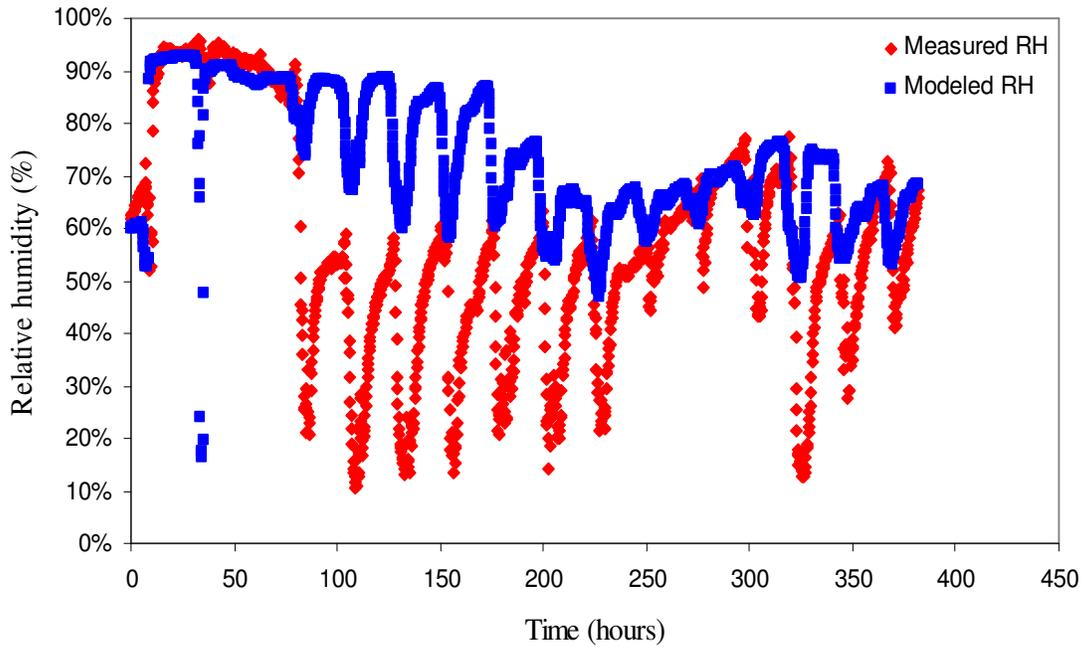
Figure 7. Measured and modeled RH data for the drained and ventilated wall 17.
