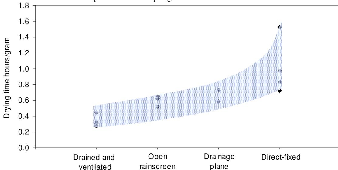
Figure 9. Summer drying rates from the water managed cavities in 22 experimental walls with absorbent wall claddings.
