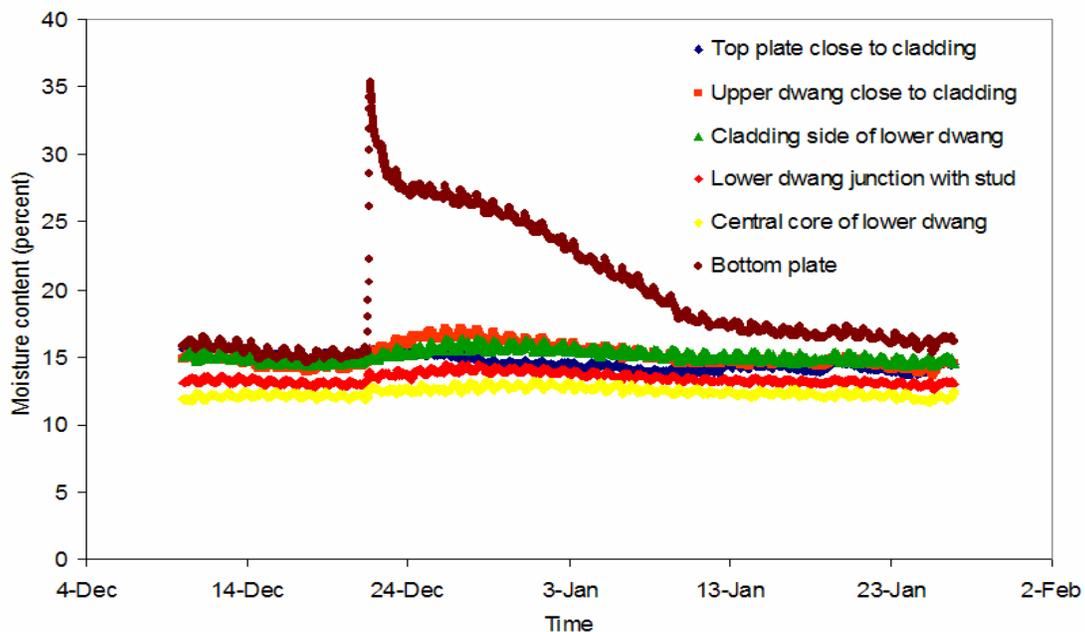
Figure 10. Timber moisture contents in wall 7, evidence of water tracking through the wall wrap in a direct-fixed wall.
