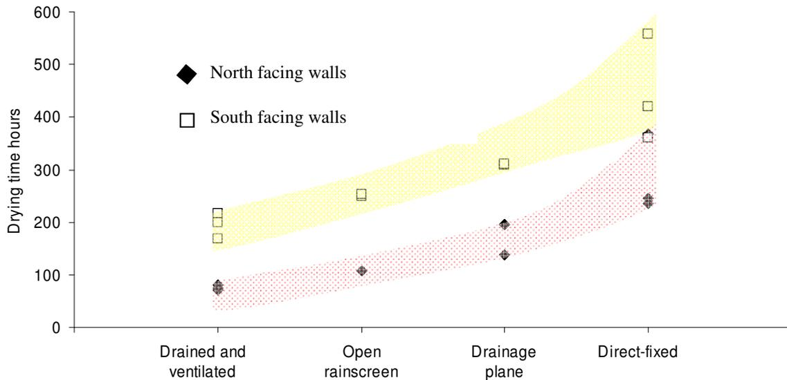
Figure 3. Year average drying times from the insulated spaces of walls facing north and south.
