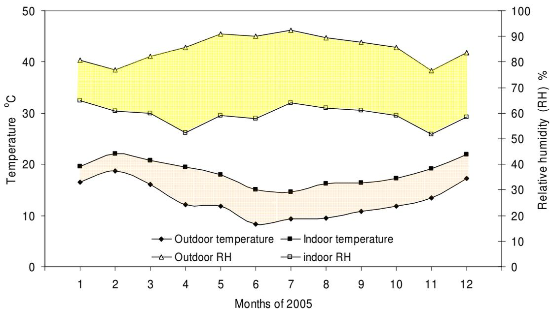
Figure 2. Average temperatures and RH inside and outside the experimental building.
