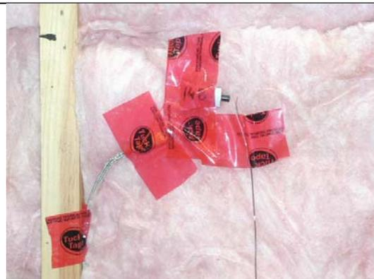
**Figure 17 - Close-up of sensors located on polyethylene membrane (inside) - Location 3**
