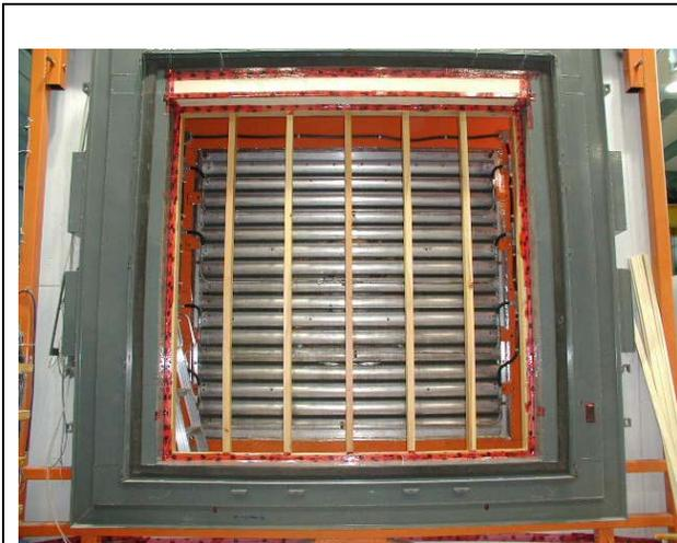
**Figure 10- Installation of the wood-stud frame in EEEF**
