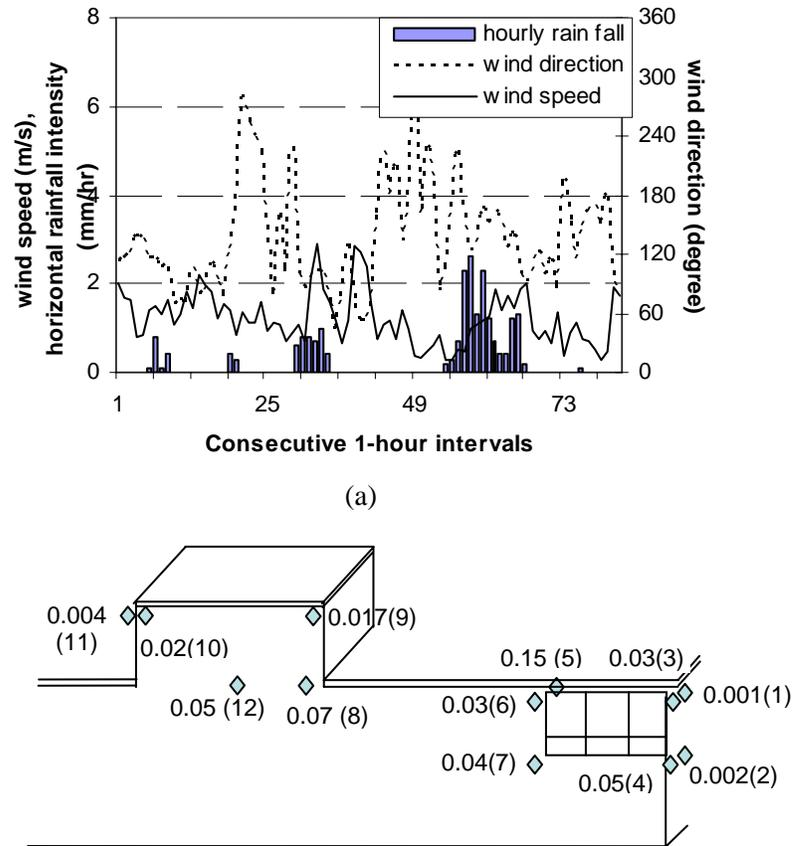
Figure 9. Measurement results for the rain event from March 30 to April 2 2006. (a) hourly horizontal rainfall intensity, wind speed, and wind direction (averaged on a 4-minute basis). Total horizontal rainfall of 21.6 mm. (b) Spatial distribution of the catch ratio for this rain event (gauge number is shown in brackets).
