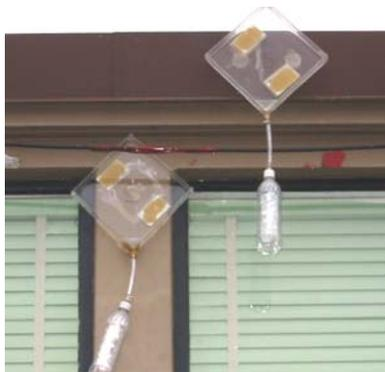
Figure 4. Driving rain gauges installed on the east face of the building.
