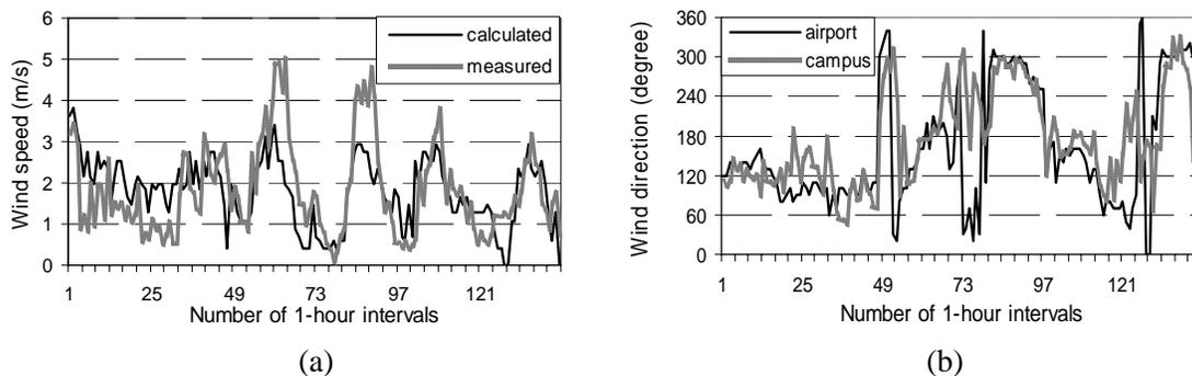
Figure 7. Rain event from March 22 to March 27. (a) comparison in wind speed between on site measurement and estimation using airport data; (b) comparison in wind direction between on site measurement and that recorded at the airport.
