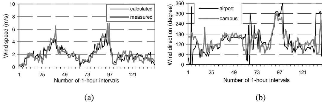
Figure 6. Rain event from March 5 to March 10. (a) comparison in wind speed between on site measurement and estimation using airport data; (b) comparison in wind direction between on site measurement and that recorded at the airport.
