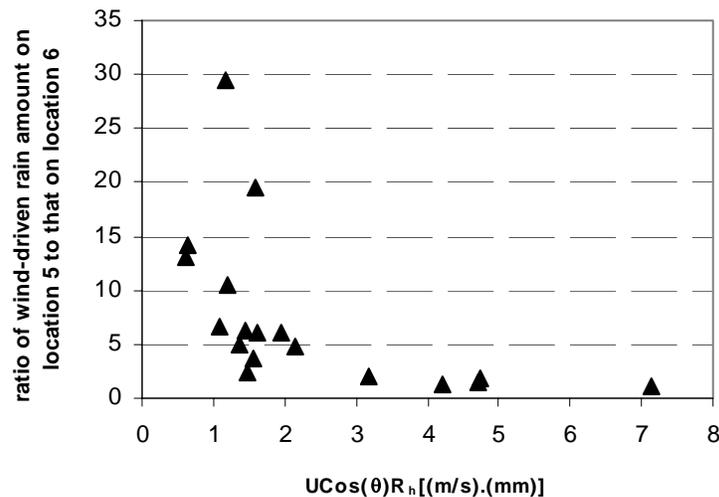
Figure 10. The effect of overhang in reducing wind-driven rain as a function of the rain and wind characteristics.  $U$  is the wind speed measured at 10 m above ground (m/s),  $\theta$  is the angle between wind and the normal to the wall, and  $R_h$  is hourly horizontal rainfall (mm).
