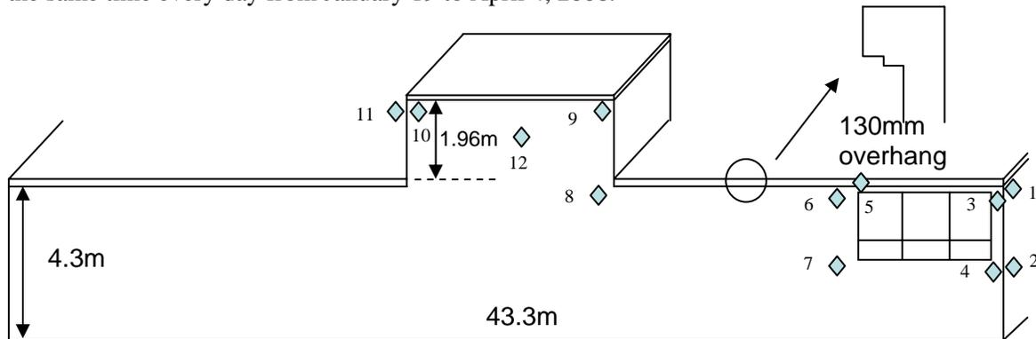
Figure 3. Building geometry and locations of driving rain gauges (not to scale).
