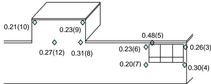
Figure 12. Wall factors on the east wall surface (gauge number is in the brackets).
