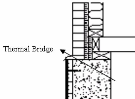
Figure 2. Typical Foundation Wall/Above-Grade Wall Interface
