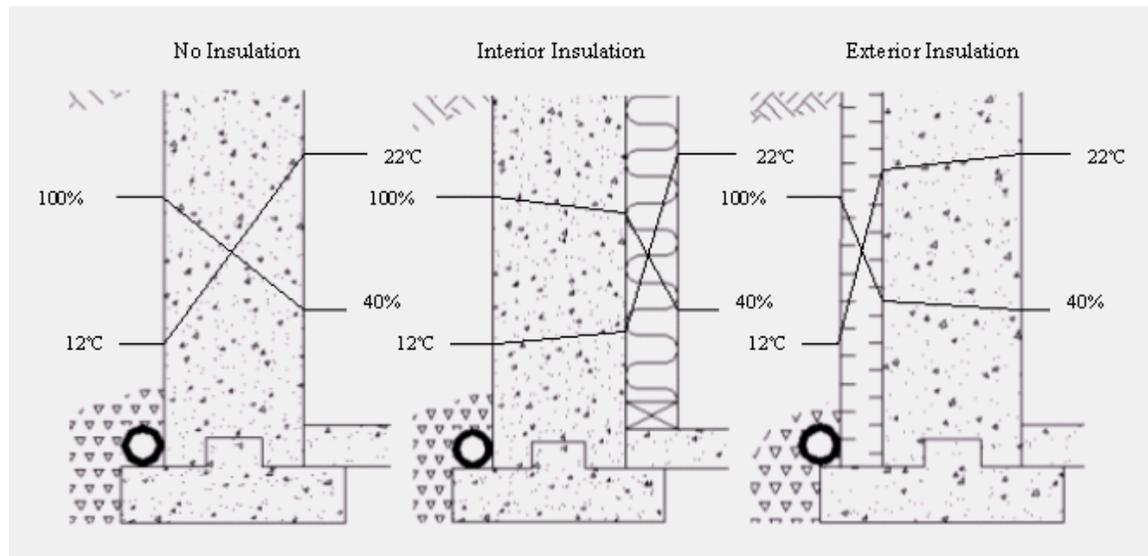
Figure 1. Temperature and Humidity Profiles for Three Wall Designs:
