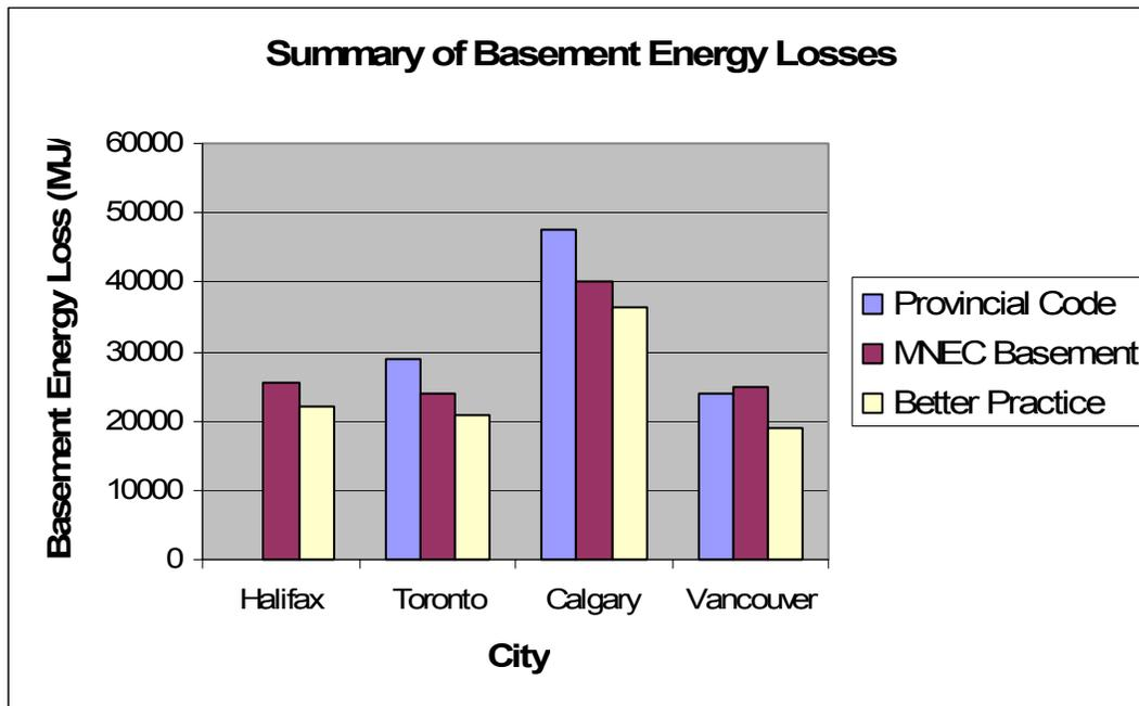
Figure 3. Basement Heat Loss by Location and Scenario
