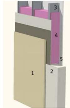
Figure 10. Isometric view of Stucco clad concrete and steel stud assemblies
