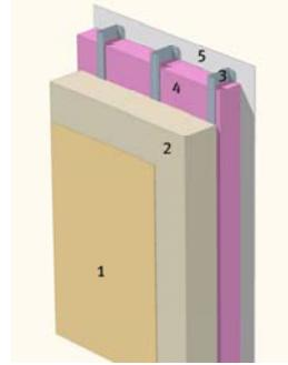
Figure 8. Original coated concrete wall assembly
