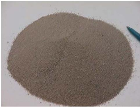
Figure 6 - Hydrophobic aggregate
