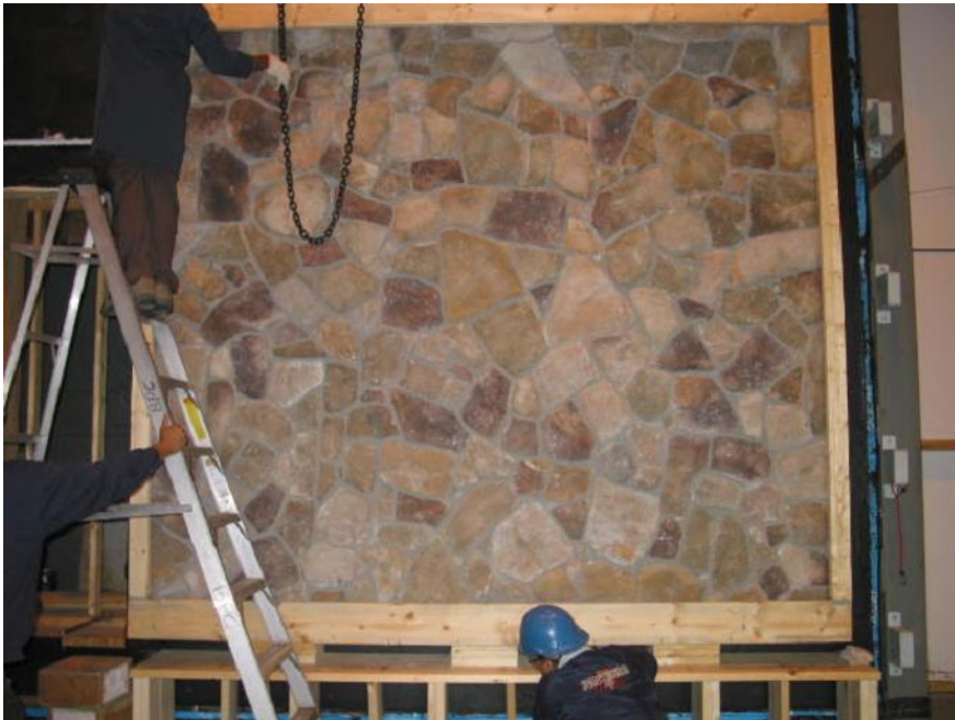
Photograph #7 – Panel mounted against test chamber
