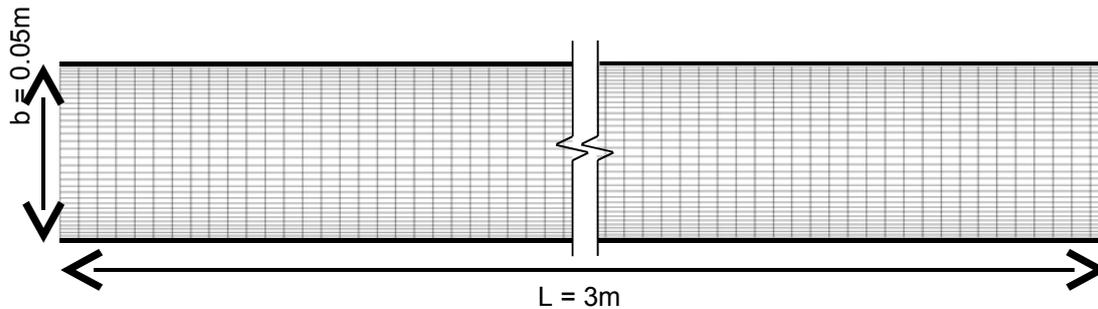
**Figure 2. Initial mesh used for the laminar CFD simulations (19,800 elements).**
