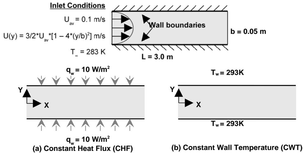
**Figure 1. Schematic representation of the two laminar case studies with (a) constant heat flux or (b) constant wall temperature**
