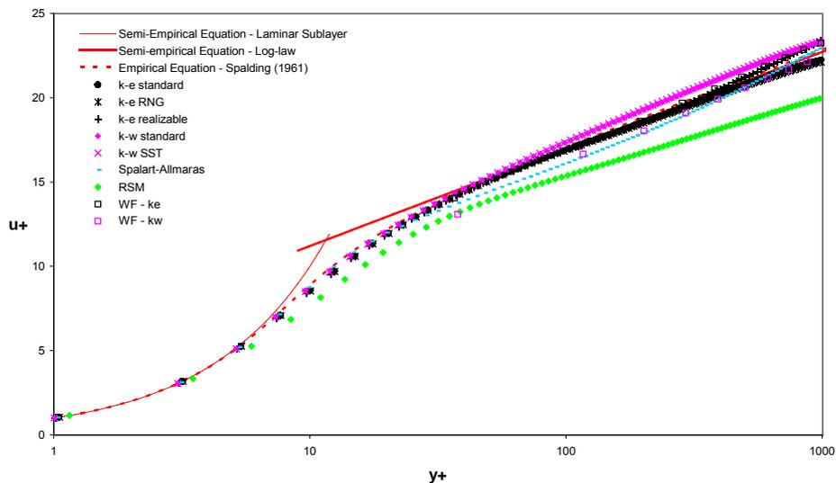
Figure 8. Dimensionless velocity profile results for the turbulent simulations
