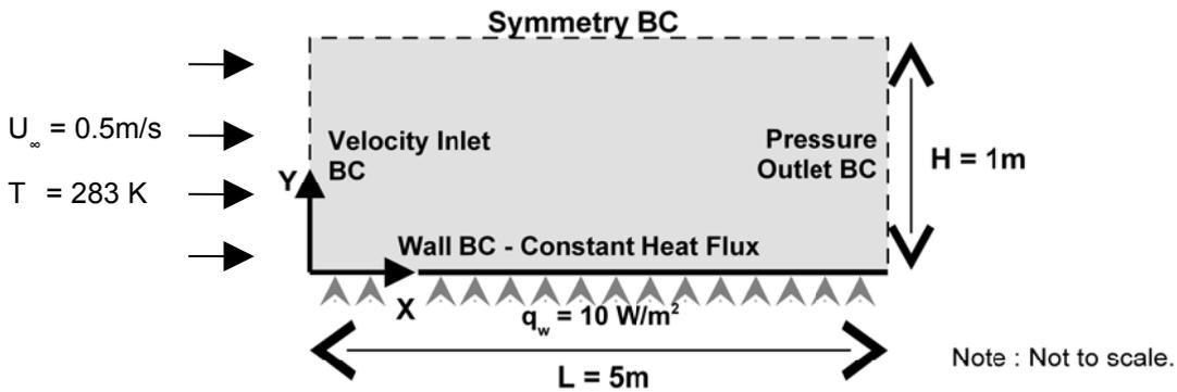
Figure 6. Computational domain and boundary conditions (BC)
