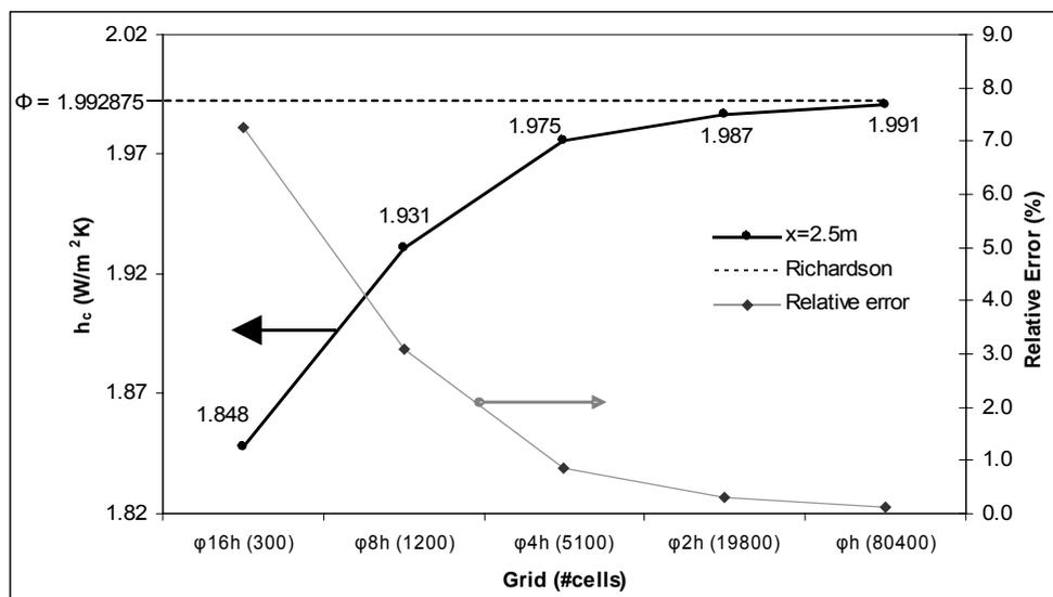
Figure 4. Grid convergence of the heat transfer coefficient for constant heat flux and relative error compared with Richardson solution
