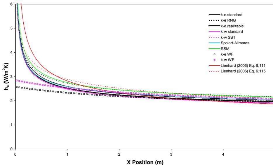
Figure 9. Convective heat transfer coefficient results for the turbulent simulations
