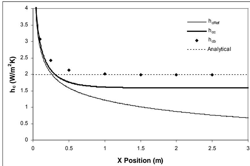
Figure 3. Convective heat transfer coefficients for constant wall heat flux
