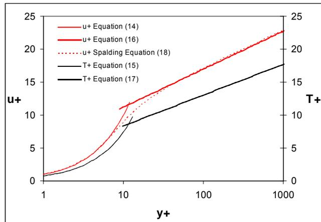
Figure 5. Wall function dimensionless velocity and temperature distributions
