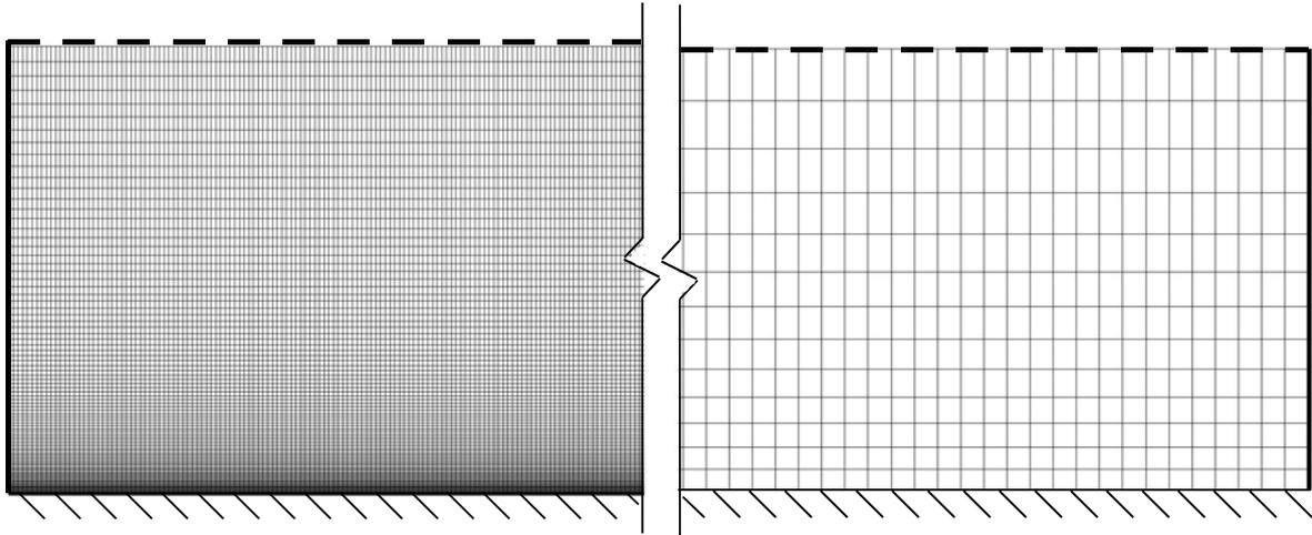
Figure 7. Grids used for low-Reynolds-number modelling (left) and wall functions (right)
