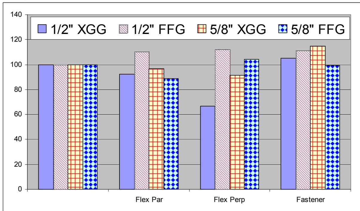
**FIGURE 4. TEST RESULTS FOR RE-DRIED GYPSUM SHEATHING**
