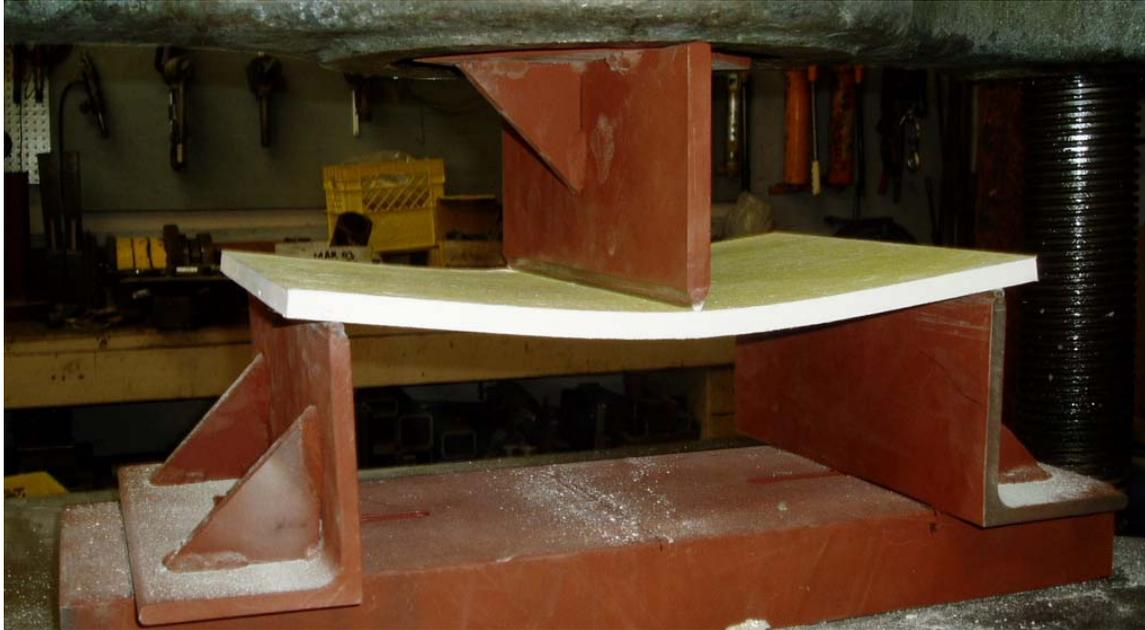
**FIGURE 1B. TESTING APPARATUS FOR FLEXURAL STRENGTH**
